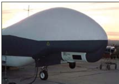
▲ Fig. 5 EHEP sensor on Global Hawk UAV (photo: EADS).
