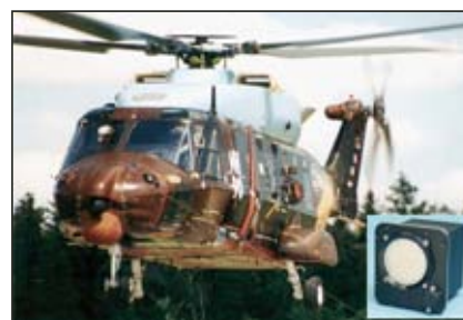
▲ Fig. 7 MILDS AAR-60 missile warner in the NH90 configuration (photo: EADS).
